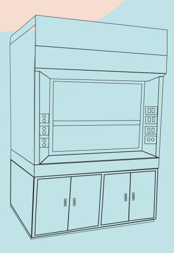
A laboratory fume hood is a ventilated, enclosed workspace designed to protect users from exposure to hazardous fumes, vapors, and dusts generated during laboratory experiments. It functions by drawing air and contaminants into the hood, capturing and exhausting them through a ventilation system, preventing them from spreading into the laboratory environment.
